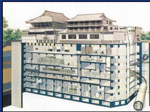
Underground substation construction
